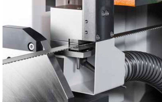
Prepared for suction unit.
