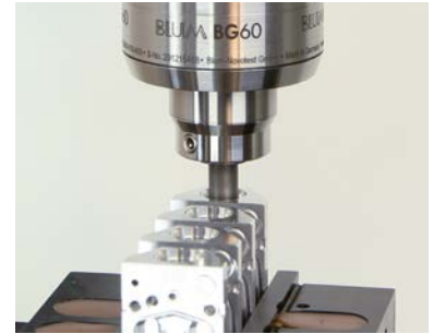
Diameter Measurement with BG60
